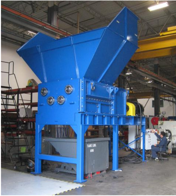
BTT incorporates robust features such as SSP™ (Severe Shock Protection), enabling systems to process tougher materials such as metals.
